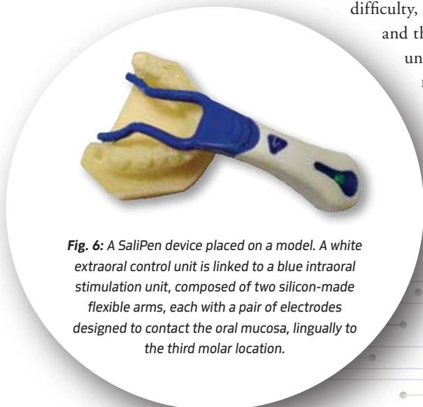
**Fig. 6:** A SaliPen device placed on a model. A white extraoral control unit is linked to a blue intraoral stimulation unit, composed of two silicon-made flexible arms, each with a pair of electrodes designed to contact the oral mucosa, lingually to the third molar location.
