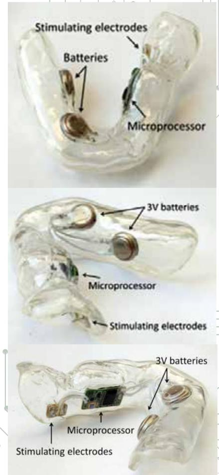
**Fig. 3:** The Saliwell device seen from above (Fig. 3a) and from both sides.
